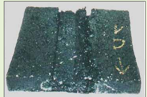
Formation of a rut without EcoStab-7
